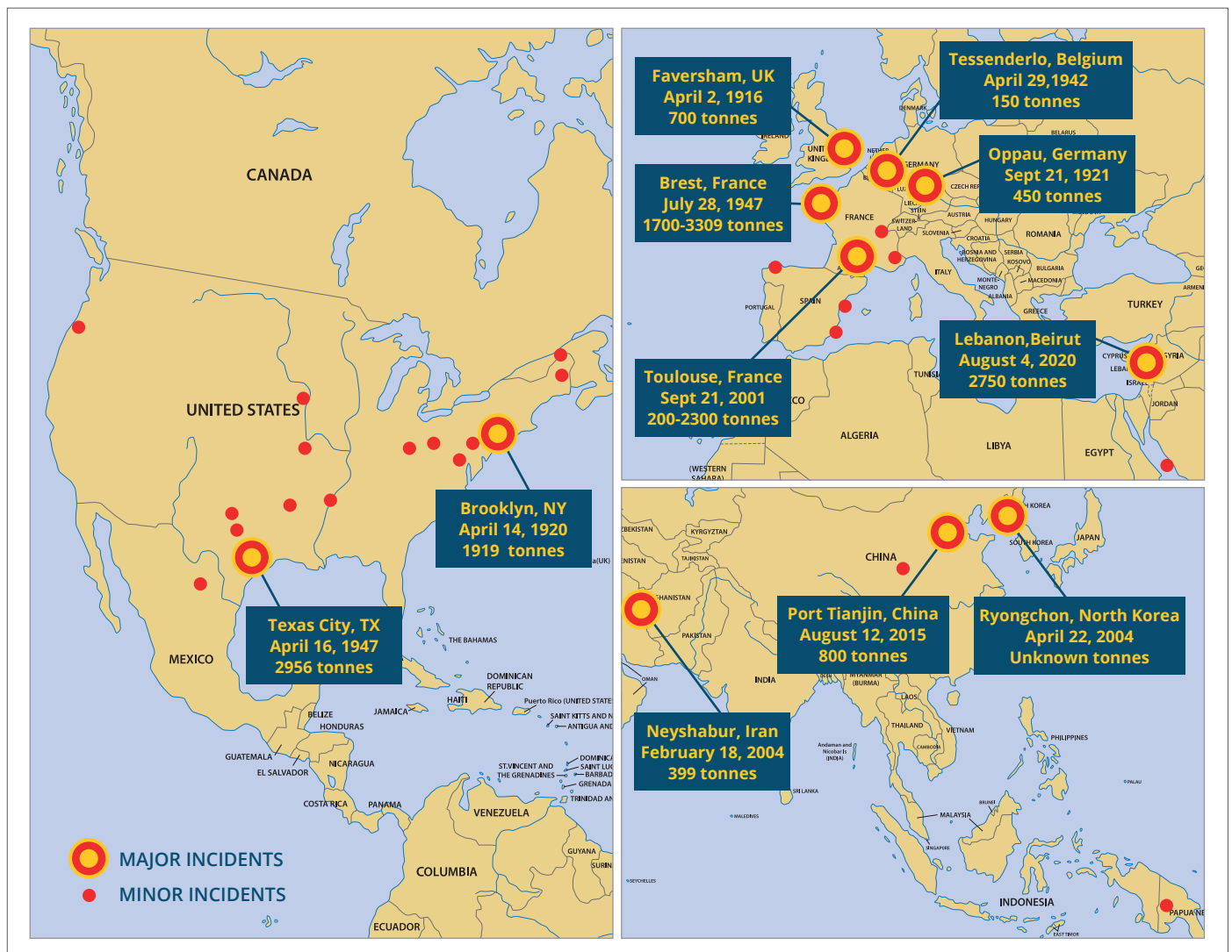
Figure 1. Accidents of ammonium nitrate around the globe. Major accidents are those that involved more than 1,000 tonnes of AN or caused more than 30 deaths during the explosion (Five of the minor accidents are not shown in the figure).
